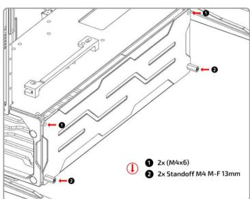
Install the PSU Top Shroud onto the PSU Mount and PSU Front Shroud using 4x M4 x 6mm.
