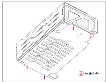
Install the PSU Side Shroud using 2x M4 x 6mm fasteners at the top and 2x Standoff M4 M-F 13mm at the bottom.
