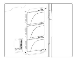
2) PSU Top Shroud. x2 2.5" drives can be installed in this location only if vertical GPU mounts are not being used.
