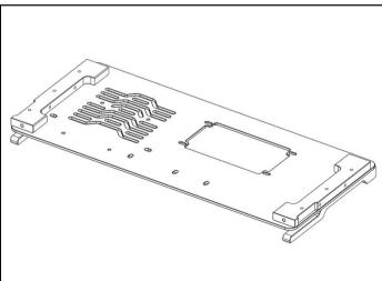
Attach the Vertical GPU Mount to the bottom panel in the position marked in diagram below using x2 M4 10mm Fasteners.
