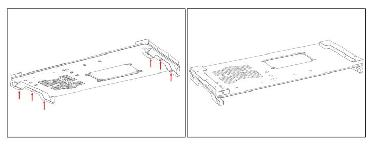
Attach Vertical GPU Mount to bottom panel in the position marked in the diagram below using x2 M4 6mm fasteners.
