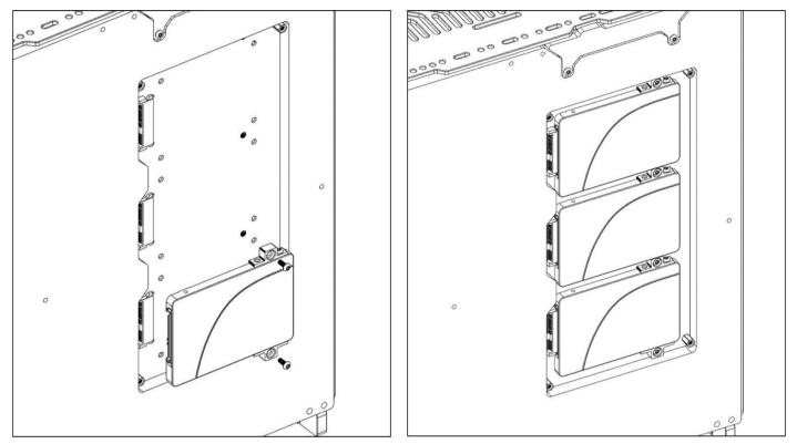
On the bottom panel of Wraith there is a 2.5" and 3.5" drive mount.
